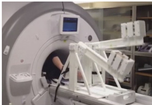
Fig. 1 MRI-compatible exercise device. The subject exercises in the magnet bore via a dynamic stepping motion to the beat of a metronome. Resistance is controlled by removable weights at the end of each lever
