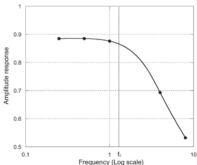
**Fig. 6** Dynamic response of a microfluidic system. This plot demonstrates that the system behaved like an RC low pass filter with a cutoff frequency ( $f_c$ ) of 1.3 Hz. Note that for frequencies above  $f_c$ , the amplitude is reduced significantly whereas for frequencies below  $f_c$ , it is not.
