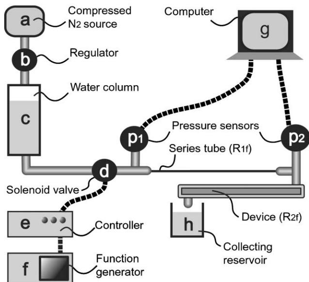
**Fig. 2** Schematic of measurement system. A compressed, dry nitrogen gas source (a) connected to a regulator (b) was used to pressurize a water column (c). Between the water column and the system outlet were a solenoid valve (d) for controlling pressure, a glass tube acting as a series resistance and a microfluidic device.
