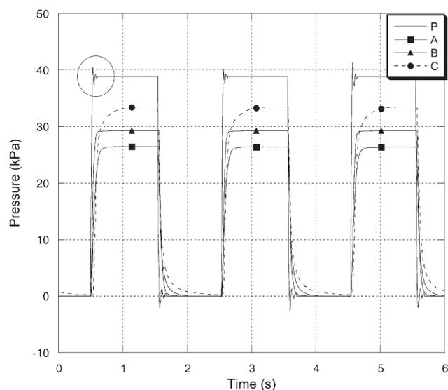
**Fig. 3** Response of the system (P) and three microfluidic devices (A, B and C) as in Table 1) to dynamic step changes in pressure. All devices showed delayed rise times which could be used to compute the compliance of devices ( $C_{2f}$ ) according to eqn (2). Note, line P is unstable at the rising edge of each step (see circled region). To determine the source of the oscillation, a balloon popping test was performed<sup>25</sup> and the result suggested that sensor error was responsible.
