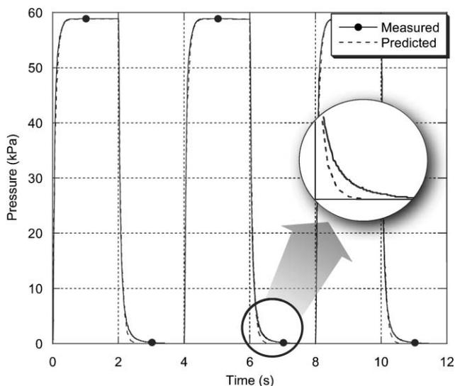
**Fig. 7** Comparison between the predicted and measured curves. The rise curves match exactly; however, there is some mismatch between the decay curves (see magnified inset of the decay curve). This mismatch is thought to be caused by hysteresis in the device, geometric non-uniformities and the non-Hookean property of the device.
