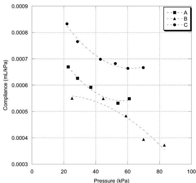
**Fig. 5** The calculated compliance of the microfluidic devices A, B, and C from dynamic step change in pressure experiments. The compliance of device C was greater than the other devices because it had a larger membrane area, despite its smaller membrane thickness. The compliance of device B, which had the thickest membrane and a membrane area less than or equal to the other devices was less than that of the other devices, as expected.
