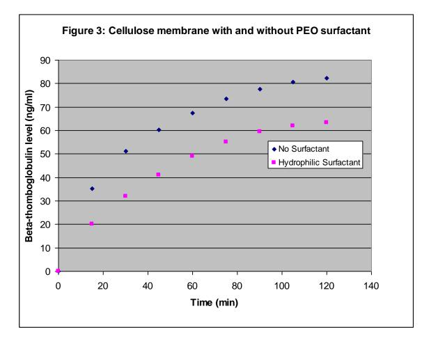
untreated membrane was 82.3 ng/ml versus 63.2 ng/ml for the blood exposed to the sample treated with PEO.
