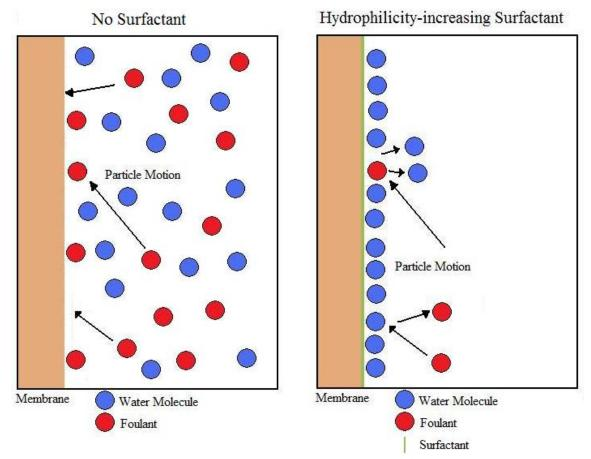
Figure 1: Foulant interaction with polymeric membrane without hydrophilic surfactant (left). Foulant interaction with polymeric membrane with hydrophilic surfactant (right).
